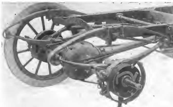
Rear Construction Displaying the Scroll Ended Springs
